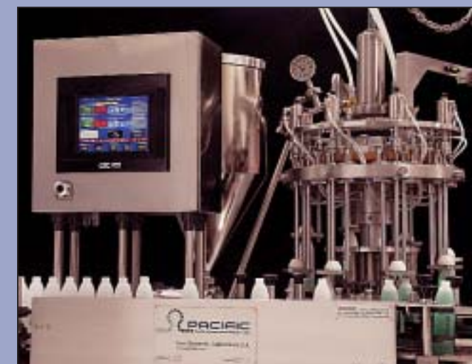
Versatile 8-station filling machine with speeds ranging from 80 to 120 containers per minute
