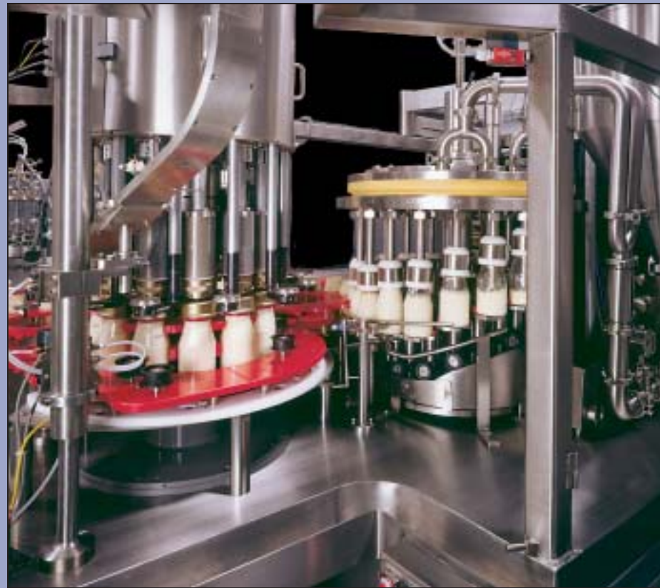
Monoblock 20-station filling turret and 12-station capping turret for viscous products
