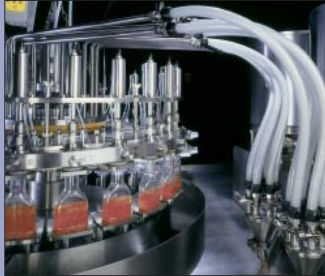
24-station two-stage pourable salad dressing filling machine
